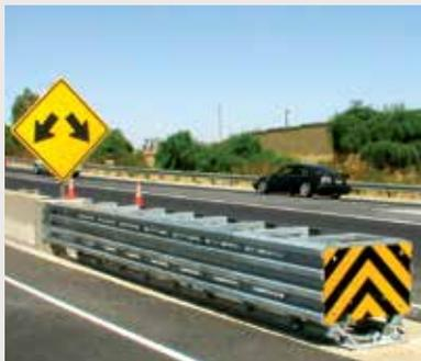
The Smart Cushion® crash attenuator is a revolutionary, speed-dependent product that varies stopping resistance during an impact. The Smart Cushion® crash attenuator allows lighter and slower-moving vehicles to have longer ridedown distances and lower ridedown g-forces.
